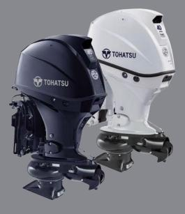
Designed for compact control, idling and trolling speed can be adjusted by pressing the key switch. (from 650 to 950 RPMs)
