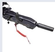
Multi-Function Tiller Handle (Option)\* Offering smooth control and easy operating keyswitch with adjustable idle speeds, big- shift handle, and tilt & trim switch on a bigger tiller handle.
