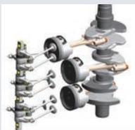
SOHC with unique 9-Valve Design with roller rocker arms provide minimal friction offering quicker throttle response more durable against wear and tear.
