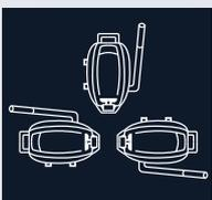
3-way storage positions (Port, Front, and Starboard side down) without worrying about oil spill.
