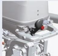
Front mounted shift lever for forward-neutral-reverse is an industry first in its class.
