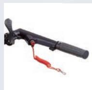
Multi-Function Tiller Handle offers the Stop Switch, Front Shift, Friction Adjusting Screw and Power Tilt Switch (PTS: on power tilt models only) integrated into the tiller handle for convenience
