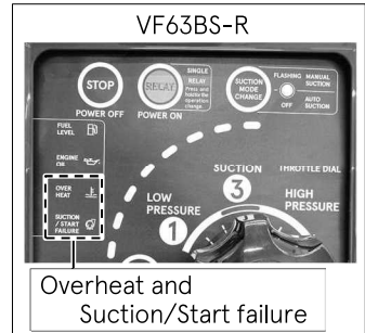
Overheat and Suction failure
